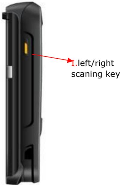
**a. Barcode scanning key:** You can scan barcodes by pressing this key.
