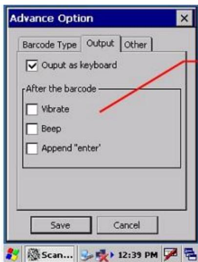
On the **Output** tab page, you can select the displayed options to send messages after bar code scanning, such as Enter event, Beep, and vibration.
