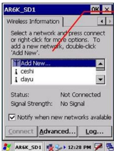
On the **Wireless Information** tab page, available networks are displayed. You can view the SSIDs of APs for which the broadcast function is enabled.
