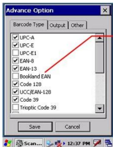
In the **Barcode Type** list box, choose bar code types for which the decoding function is enabled.
