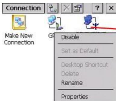
This icon is displayed only when the Wi-Fi function is enabled. Use the stylus to click and hold down the icon and choose **Properties** in the displayed context menu.
