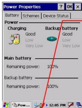
When the electricity is insufficient, the system displays a warning icon on the taskbar. You can display the **Power Properties** dialog box by clicking the warning icon.
