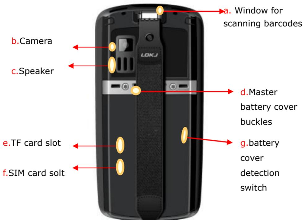
**a. Windows for scanning barcodes:** Laser comes out from this window. donot look into the window with naked eyes.
