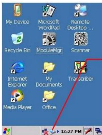
Click the network icon to display the interface for setting the Wi-Fi function.
