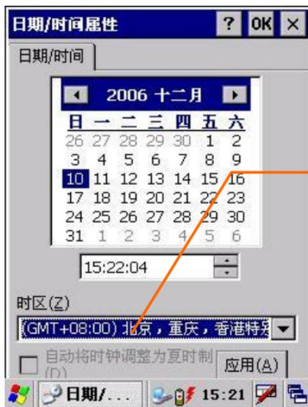
Click the Time Zone drop-down list to choose the required time zone. Click Apply on the lower right corner of the dialog box to save the configuration.
