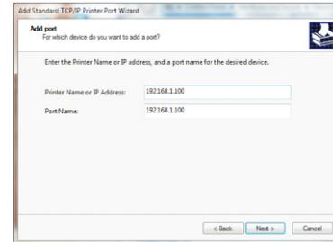
4, Add the standard TCP / IP Printer Port Wizard, select the device type, and then click "Next" to continue the installation, See the following image:
