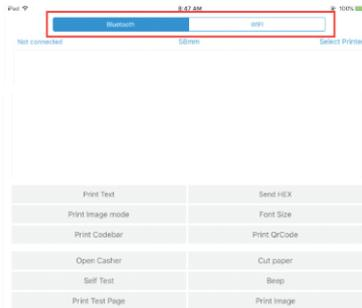
5. If connect with Bluetooth, then you can click " Select Printer" first, you will search the "Bluetooth Printer" (the default name of printer is Bluetooth Printer), click it to be connected.
