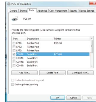
2. Select the list of ports "COM1" → "Configure Port", the printer factory default settings as shown below:
