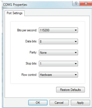
You can see the setting parameters of serial port from self-test page. Click "Apply", then click "OK" (Note: This setting must be consistent with the setting parameters of serial port from the printer self-test page, otherwise it will be garbled case) appears as shown below:
