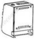
1. Remove the DIP switches cover on the bottom of the printer.
