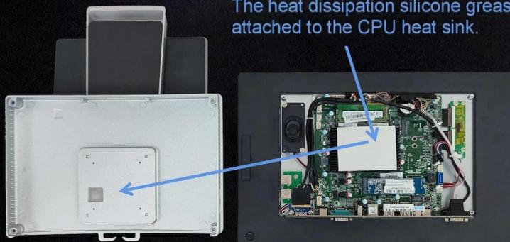
The heat dissipation silicone grease is attached to the CPU heat sink.
