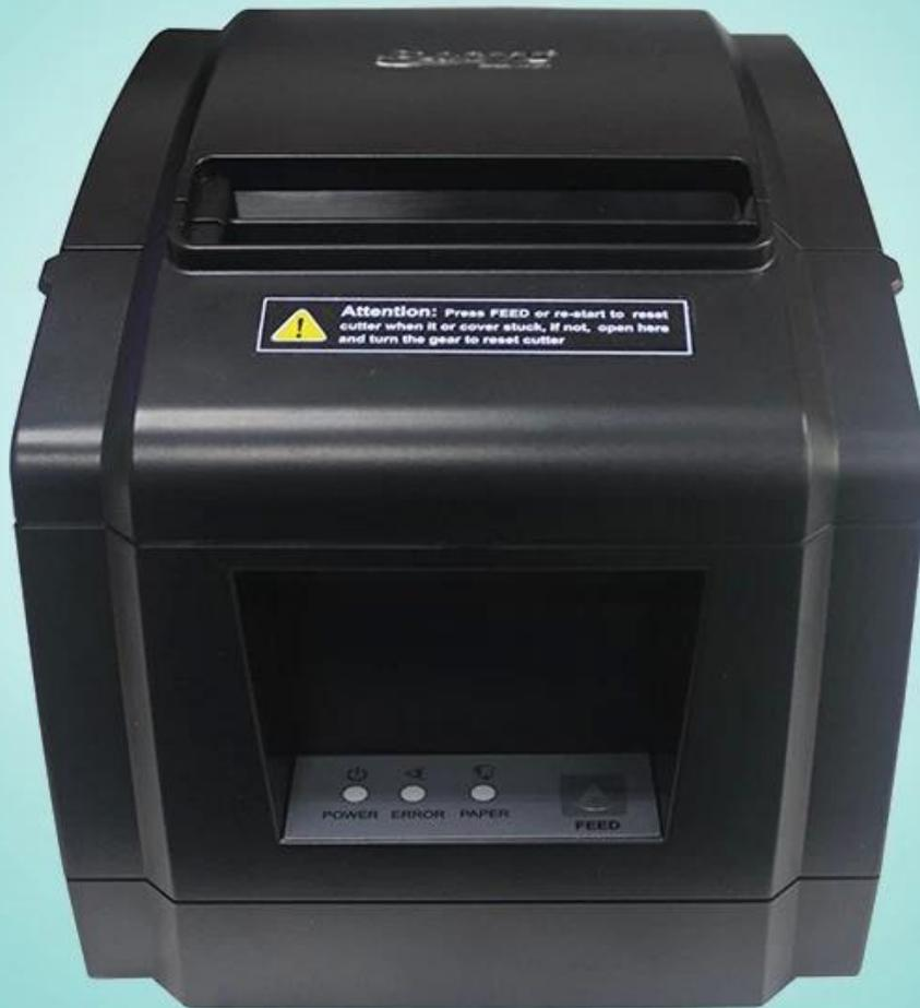
**Attention:** Press FEED or re-start to reset cutter when it or cover stuck, if not, open here and turn the gear to reset cutter
