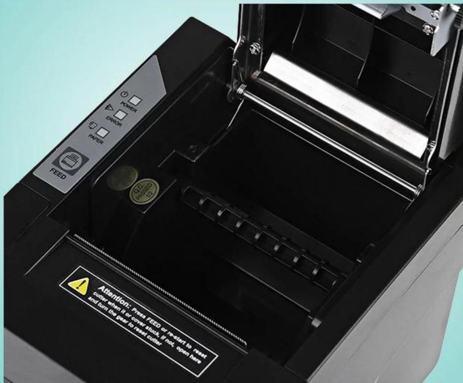
**⚠ Attention:** Press FEED or re-start to reset cutter when it or cover stuck. If not, open here
