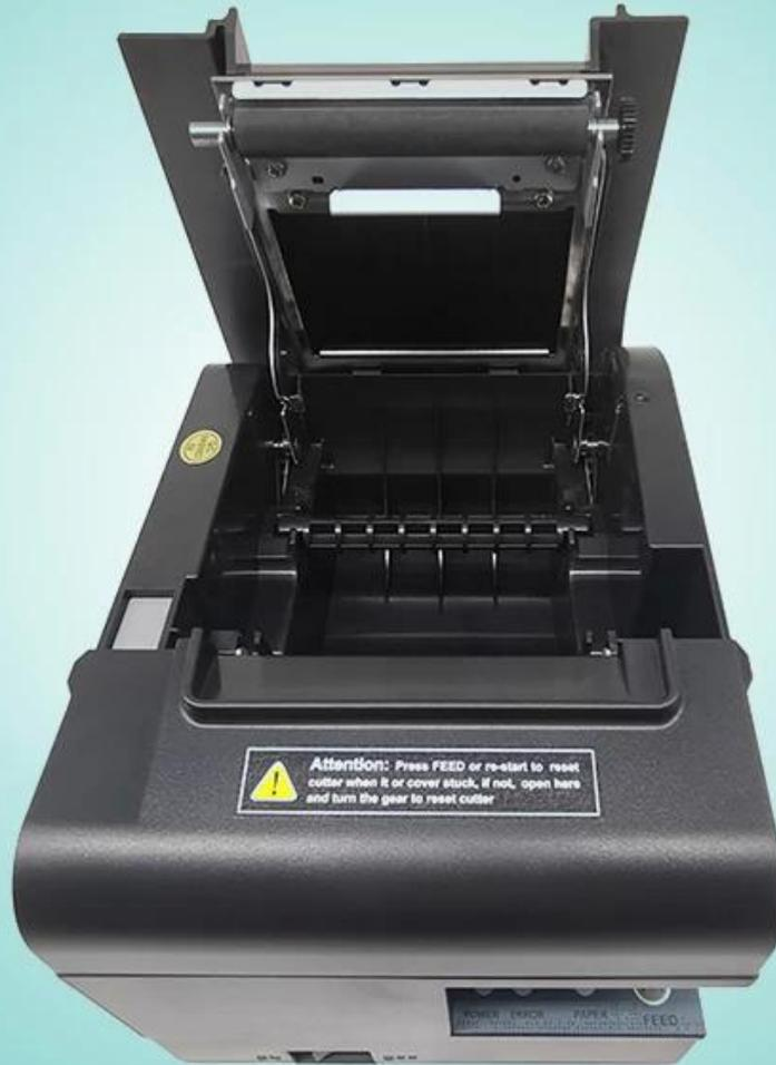
**Attention:** Press FEED or re-start to reset cutter when it or cover stuck, if not, open here and turn the gear to reset cutter
