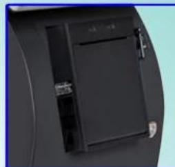
80MM thermal printer with automatic cutter
