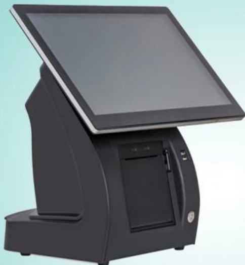
80MM thermal printer with automatic cutter
