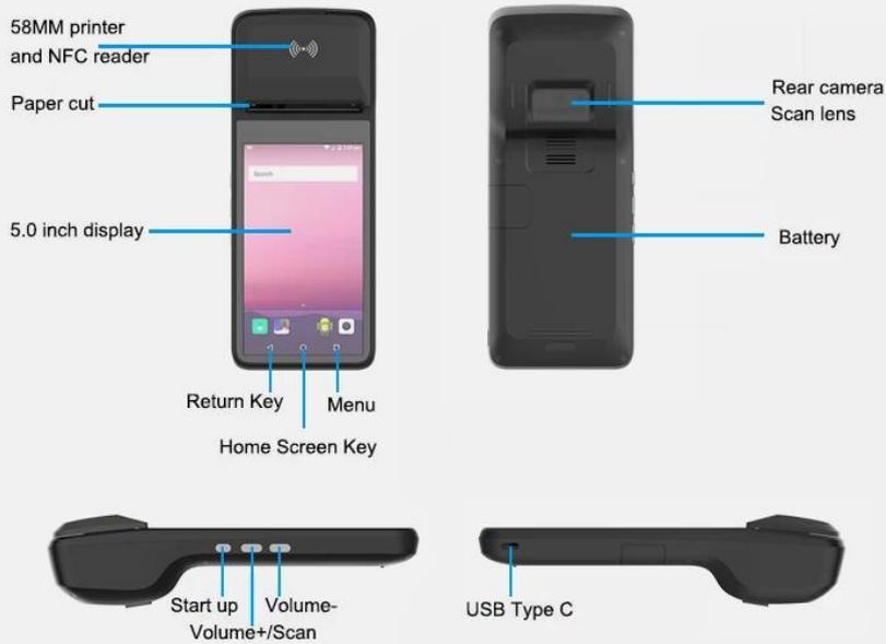
The bare weight is only 304g. The thickness of the machine is only 19.6mm, excellent grip feeling, one-hand operation is not tired, higher work efficiency.
