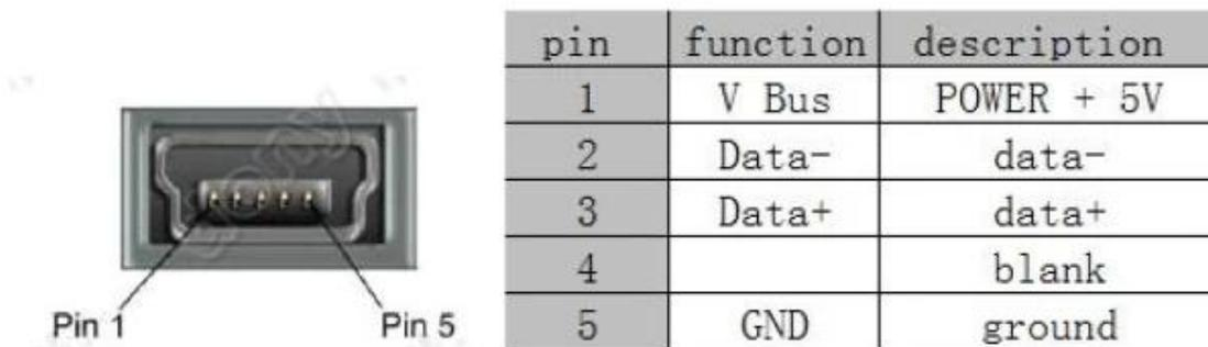
Figure 2-5; Mini-USB socket and pin definitions
