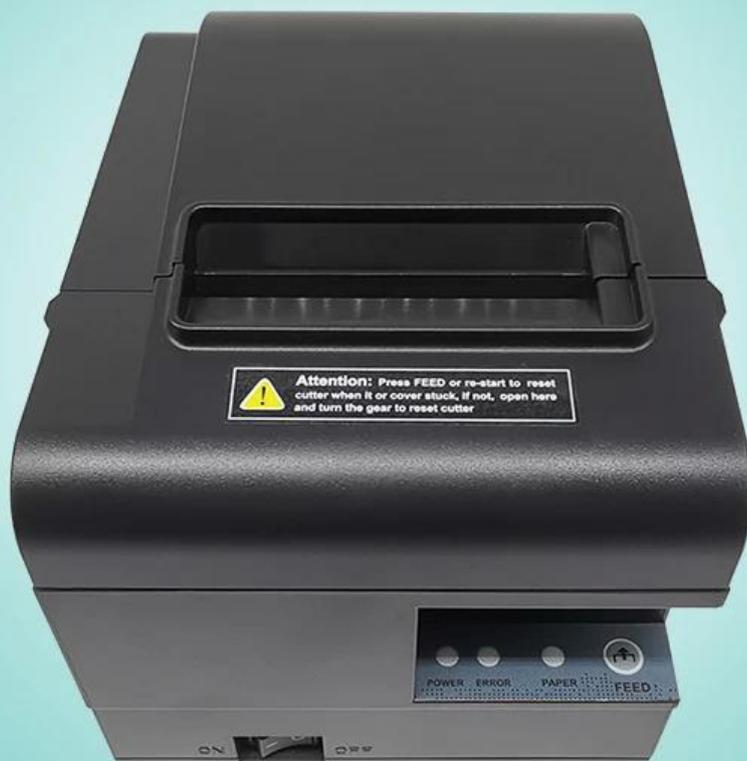
**Attention:** Press FEED or re-start to reset cutter when it or cover stuck, if not, open here and turn the gear to reset cutter
