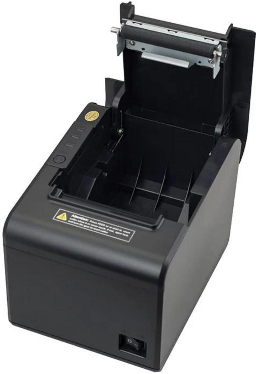
**Attention:** Press FEED to release the paper and turn the gear to reset roller.
