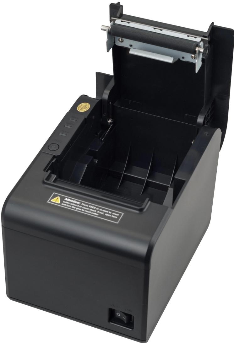
**Attention:** Press FEED or re-align the paper when it is over about 2 mm. Open the front door and press the green button to reset the paper.
