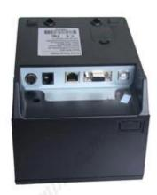
Multiple interfaces available: USB, USB+Serial, USB+LAN, USB+ Serial+ LAN; and Wifi+USB, Bluetooth+USB+LAN
