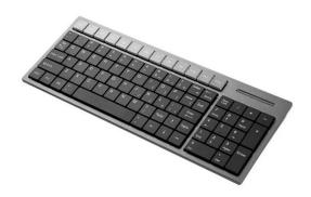
KB89 is narrow-sided, silent, membrane pos keyboard, with dust-proof andwaterproof structure; Can be divided into one-piece type and split type; also can be optional to wear the transparent keycaps&lens; Support dual-channel(USB/PS2); The color is White, black and gray. No battery required, data storage can be over than 100 years. EMC radiation reaches class B requirements, antistatic design (refer to GB4943, GB/T 17626 related standards).
