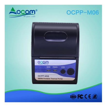
This mini printer with model number OCPP-M06 is a Android (or IOS+ Android), Window, Linux, JAVA compatible battery powered 58mm portable mobile thermal pos printer which combines USB,RS-232 Serial and Bluetooth (optional) communication ways together. This printer could be powered by rechargeable battery, power adapter, or car charger (depending on specified models). Special model can connect with 8 smart devices for printing at same time. We have CE, FCC and other required certifications.
