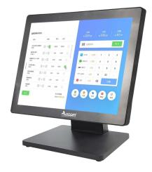
Intel Celeron series and intel core I3 I5 processor for option; Rockchip high speed RK3288 processor for option; EMMC 8GB/16GB/32GB for option; Hard Driver Msata SSD 64GB, SSD 128GB an 256 GB for option; Multi-point projected capacitive touch panel; Optional side MSR and VFD220 customer display mounted to back cover; Ture flat and water-proof scratch-resistant surface display.
