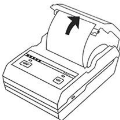
Step two Load roll paper according arrow direction
