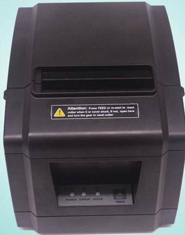
**Attention:** Press FEED or re-start to reset cutter when it or corner stuck. If not, open here and turn the gear to reset cutter.
